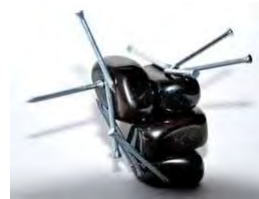
Magnetite (lodestone): \mu_0 M_s = 0.56 T ferrimagnetic
